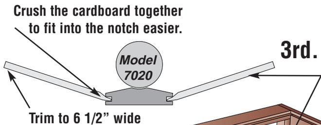
The reflector cards, as shipped, are too wide for the 7020 fixture and must be trimmed from 6 7/8" down to 6 1/2"... after trimming... crush the edge of the cardboard so it will be easy to fit into the notch on each side of the fixture's base.
