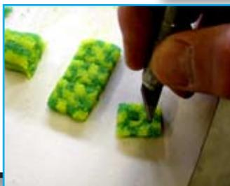
LSM has an extended working time and once it is mixed with frit and kept in an air tight container, your mixture will remain workable for many months. I have a squeeze bottle with LSM and frit that is still workable after 10 months in storage.
