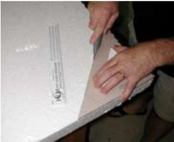
The ramp is easy to make. I just cut a piece of 1 inch thick or is thicker Styrofoam at a 45° angle and tape a smooth surface, such as a plastic ruler or a piece of glass onto the angle slide of the ramp. A ruler is handy, because it gives you accurate measurement on how much your tests sample moves over a given period of time. If you take the time to make a simple ramp and test the consistency of your paste, you will have a much higher success rate.
