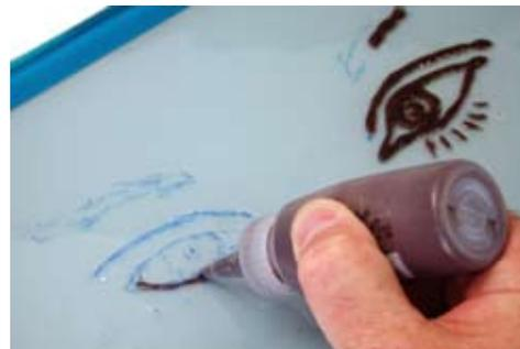
If you are having problem getting the LSM and frit paste to flow easily out of your squeeze bottle, you may have to cut the tip to slightly enlarge the opening. A #4 or larger cake decorators tip seems to work well. A #4 hole should just accommodate the tip of your average ball point pen. (1.8 mill)
