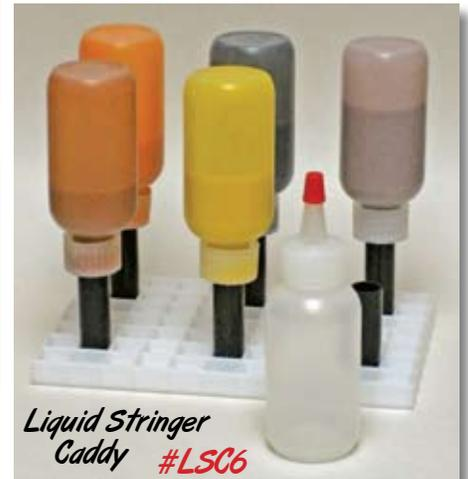
If your LSM and ground glass is not flowing from the bottle end, you may need to clean or enlarge the opening. Ream the tip with a 1/8" drill bit first. If a larger opening is needed use the next drill size larger to ream the tip.
