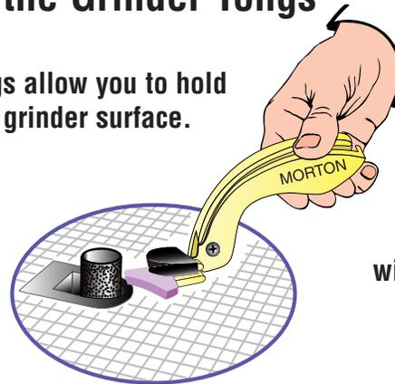
Increase gripping pressure and control while grinding by pressing down on the black rubber pad with the index finger of your opposite hand.
